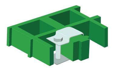
These are used for connecting unsupported butting flooring panels and are a C shape that pushes onto the end bars of the panels, and an M6 stainless screw (included) is inserted and tightened into a threaded boss. The connector is designed to eliminate potential trip hazards which could be caused by deflection when moving from one panel to another.
