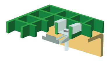
These L-shaped clips are designed to pick up on the underside of the flooring supports, eliminating the need for drilling & making them ideal for use where access to the underside of the flooring is difficult to tighten a nut. The clip works in conjunction with the saddle clip and uses a longer bolt and a square nut that is prevented from turning by the U shape of the underside of the pressing.
