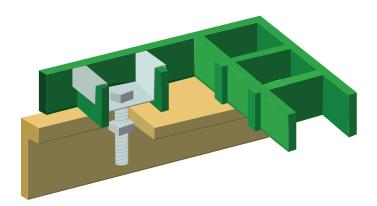
These are an M-shaped 316 stainless-steel pressing that fits over the bearing bars of the open-mesh grating. It has a 9mm central hole into which an M8 bolt is inserted and fixed to the support work with a nut and washer on the underside.
